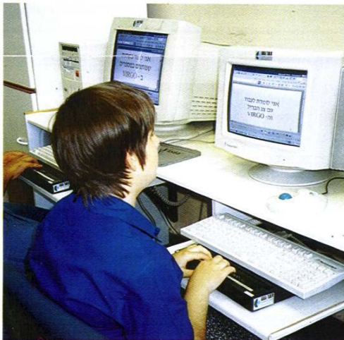
Computer usage for the blind is possible with the use of a Braille display keyboard
